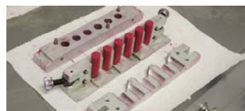
Figure 4. The lipsticks coming out of the moulds.
