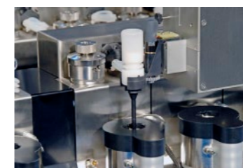
Overhead gravimetric dispensing of solid while mixing, heating and cooling in the precision formulation vessel
