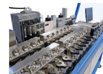
Example of a tray configuration with 24 precision formulation vessels (up to 36 precision formulation vessels), 3 gravimetric overhead dispensing robotic tools, a variety of racks with vials, syringes, heated and disposable pre-formulation vessels and much more...
