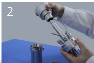
2 Mount cylindric magnetic stirrer drive
