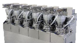
Process development workstation for 6 X 100 mL, 3 X 250 mL, 3 X 1'000 mL
