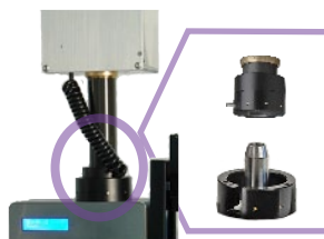
Robotic tool exchange interface (proprietary)
