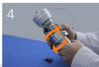
Screwless closing and self-sealing of reactor
