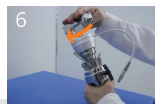
Screwless mounting and self-sealing of multiport drawer valve
