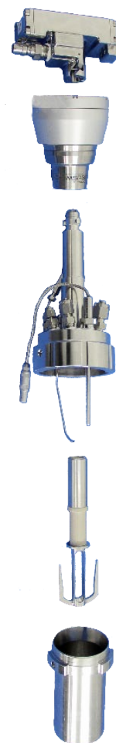
Process research reactor
